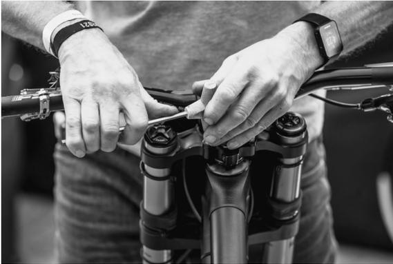
Install the lower crown & steerer into the headset, attaching the upper crown and stem to the steerer tube. Preload the top cap and tighten the clamp bolts. Clamp the stanchions through both crowns.
