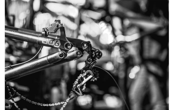
Fasten the dérailleur to the hanger, ensuring that they are aligned correctly (with b-tension screw in contact with the dérailleur's plastic washer rather than the hanger itself).
