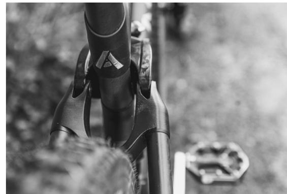
Fit the pedals of your choosing. Please note: the non-driveside pedal has a left-hand thread (removes clockwise, installs counter-clockwise).
